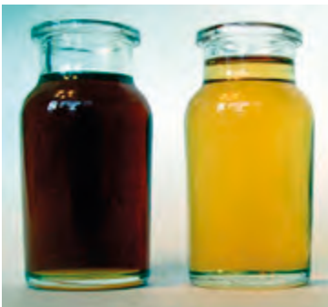
Figure 11: Degraded hydraulic oil compared to new oil Source: C.C.JENSEN A/S
