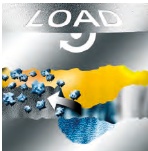
4. Surface fails + created particles
